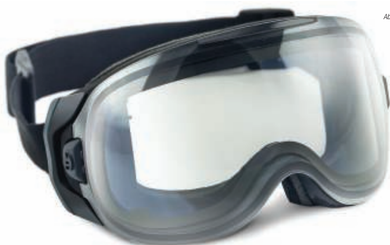
FIGURE 4. Abom's safety goggles feature inner lens surfaces that are scratch-coated and have a transparent, thin-film conductive layer through which a small current is introduced and produces enough heat to clear up fog in a matter of seconds
