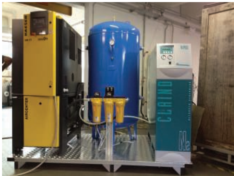
FIGURE 3. A typical onsite PSA system uses two vessels, both filled with CMS pellets. They operate in an alternating mode, so that at any time, one is in pressurization mode to enable air separation (to allow the nitrogen product stream to be collected), while the other tank is in depressurization mode, to allow the adsorbed oxygen to be released to the atmosphere (Credit: Claind S.r.l.)
