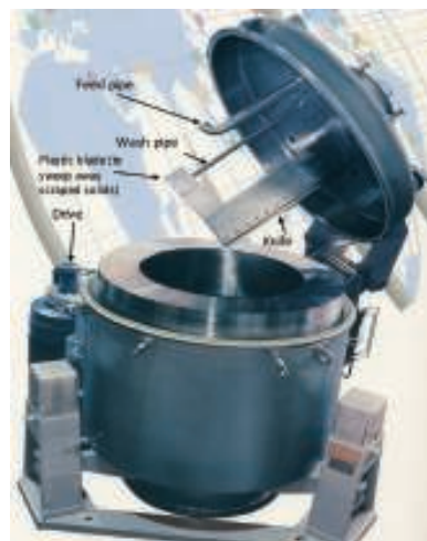
FIGURE 2. Shown here is a vertical basket centrifuge (Credit: Western States)
