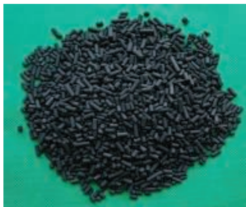
FIGURE 1. Carbon molecular sieve (CMS) pellets, typically manufactured from coconut shells, provide the surface area and pore structure needed to separate oxygen and nitrogen from a compressed air inlet stream (Credit: Comelt S.p.A.)
